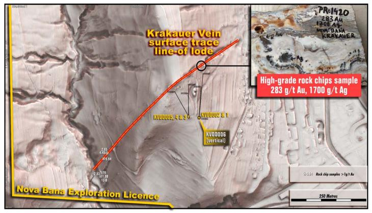
Map of the Krakauer structure showing the location of the six completed diamond drill holes.
