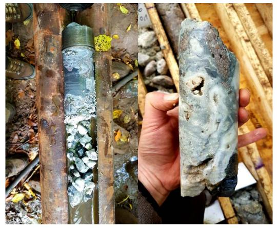
Krakauer drilling intersected brecciated quartz zones, suggesting multiple pulses of mineralising fluids. KVDD006 is being assayed at report date (depth 226m).
