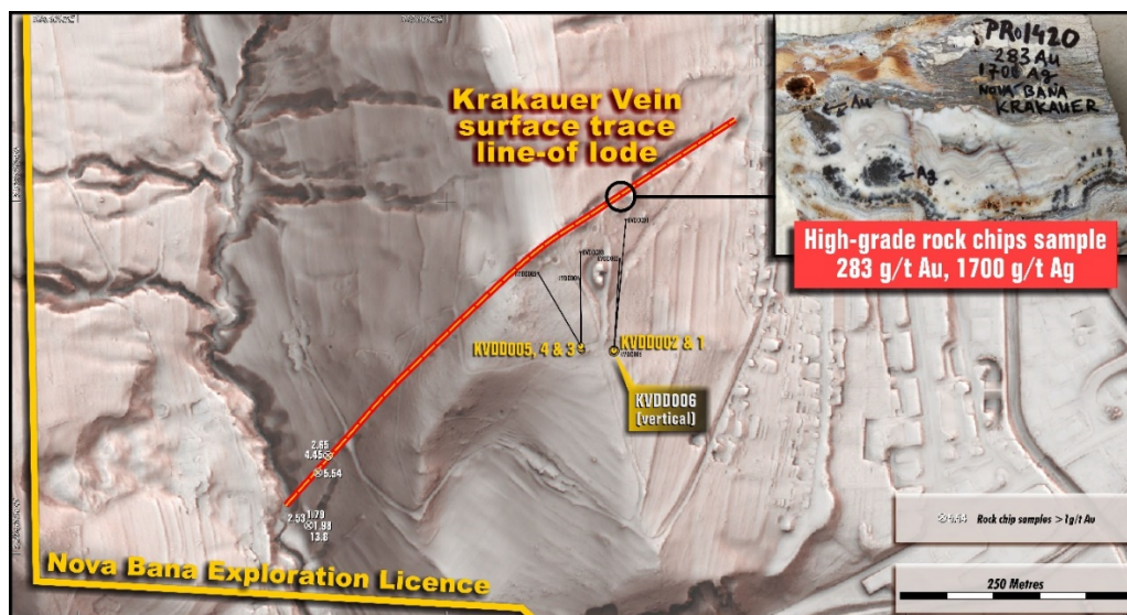
Plan view of Krakauer gold silver vein structure, which had never before been drill-tested. Shown are observed vein strike (thick red line) and completed drillholes (black traces). North is towards the top of the page.
