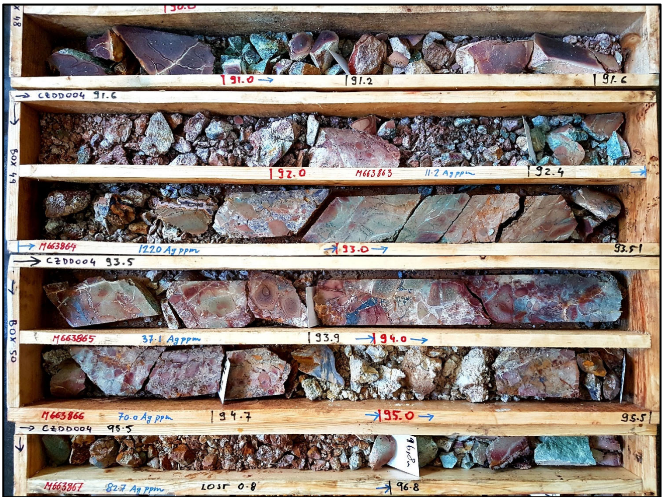
Classic banded epithermal vein from an interval in CZDD004 that assayed 1,220 g/t Ag (92.5 to 93.0m). Silver assays very similar to previous drilling with lower non material base metal intercepts
