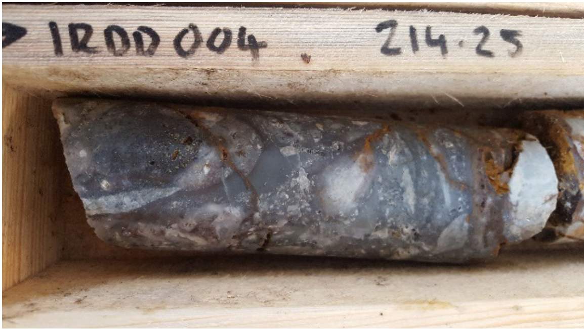
Intervals from IRDD004 contained epithermal breccias on the margins of the high grade shoot defined by holes IRDD001 and IRDD002.
