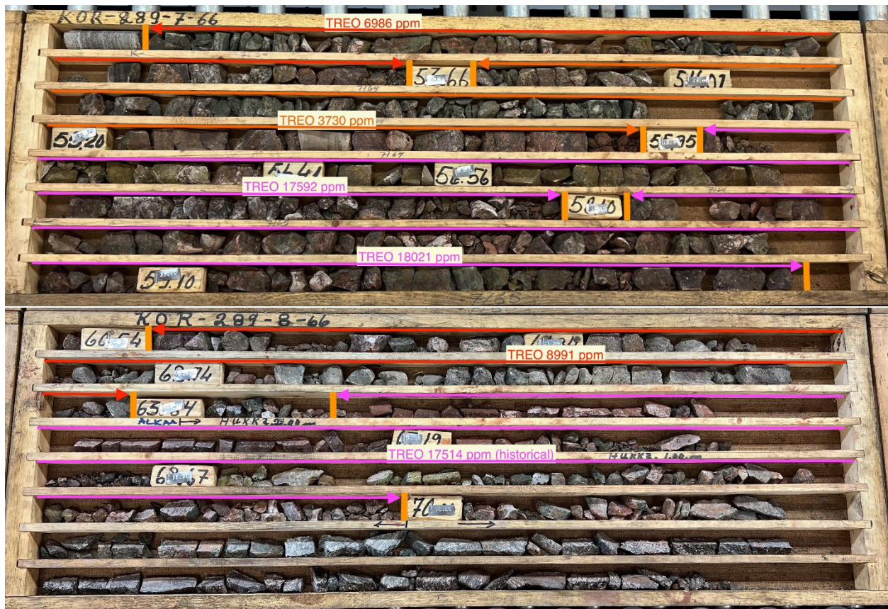
Figure 1. Photographs of hole KR-289 core with recent and historical TREO assays overlaid.
